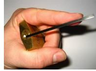
Next, insert a pick with your other hand, and push up on the pins. Try this with one of the one or two pin training locks first!
